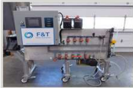
2 GPM Variable Electro Precipitation™ Commercial Test System
